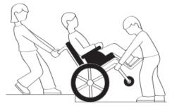
Figure 5.2: Assistant positioning for climbing curbs, for wheelchair without step tubes
