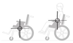
Figure 5.5: Center of gravity location
