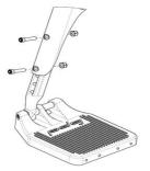
Figure 12.3: Standard Swing-Away footrest height adjustment
